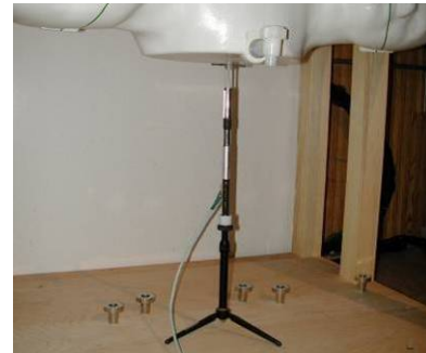
Figure 9-2 System Verification Setup Photo
