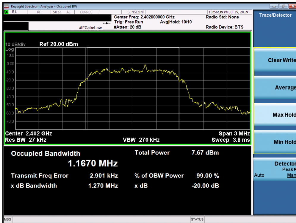
Plot 7-4. 20dB Bandwidth Plot (Bluetooth, 2Mbps – Ch. 0)
