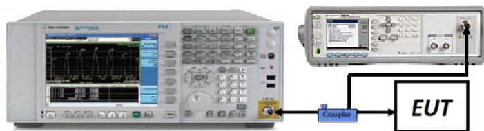
Figure 7-7. Test Instrument & Measurement Setup
