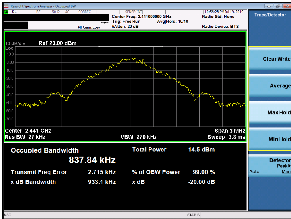
Plot 7-2. 20dB Bandwidth Plot (Bluetooth, 1Mbps – Ch. 39)
