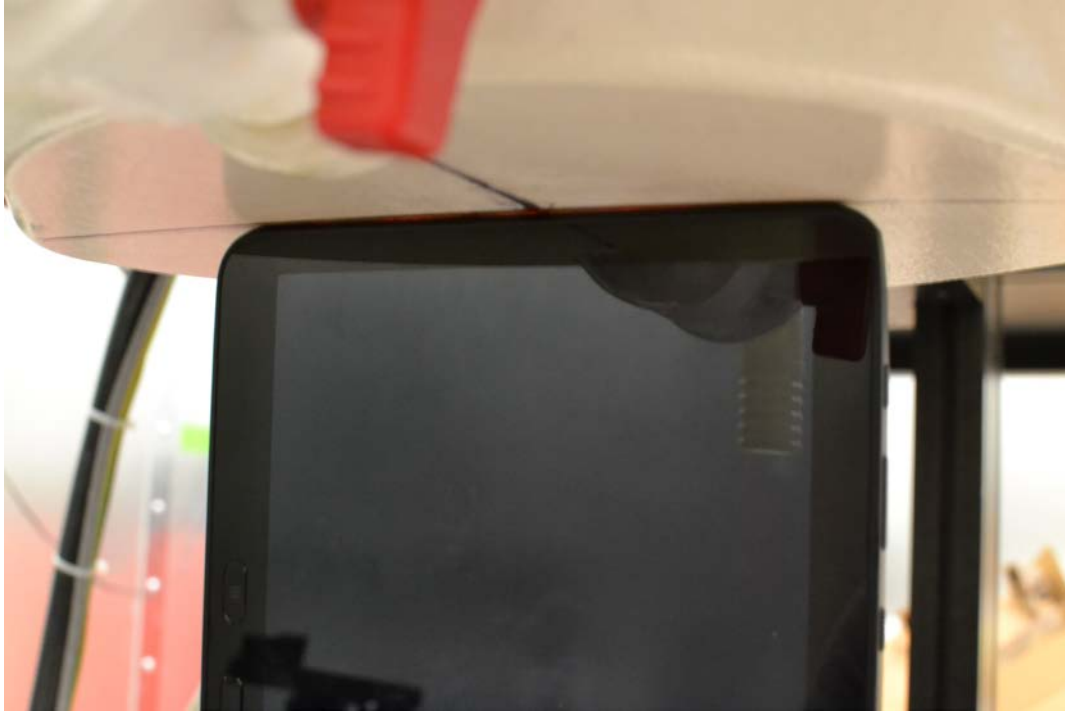
SAR Test Setup Photo 5 – Left Edge at 0 cm
