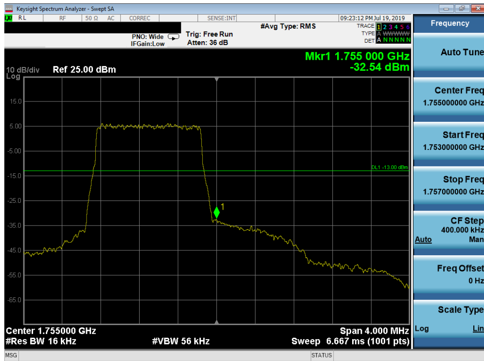
Plot 7-155. Upper Band Edge Plot (Band 4 - 1.4MHz QPSK - Full RB Configuration)
