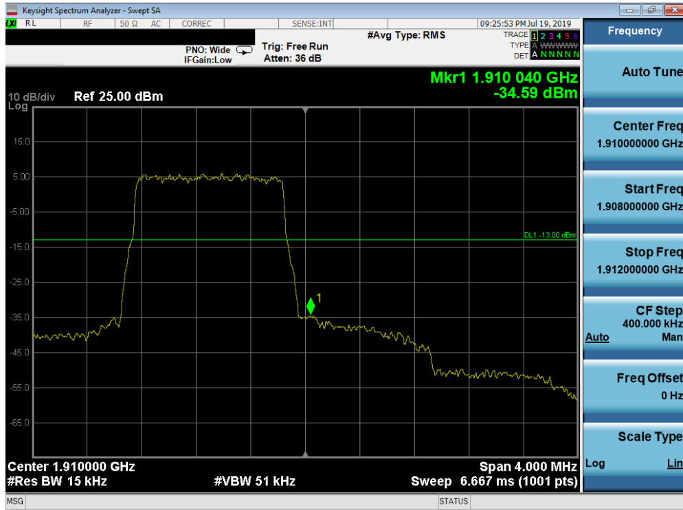
Plot 7-191. Upper Band Edge Plot (Band 2 - 1.4MHz QPSK - Full RB Configuration)
