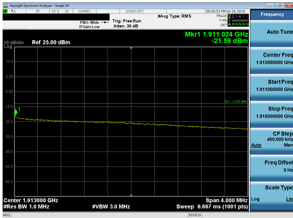
Plot 7-204. Upper Extended Band Edge Plot (Band 2 - 10.0MHz QPSK - Full RB Configuration)
