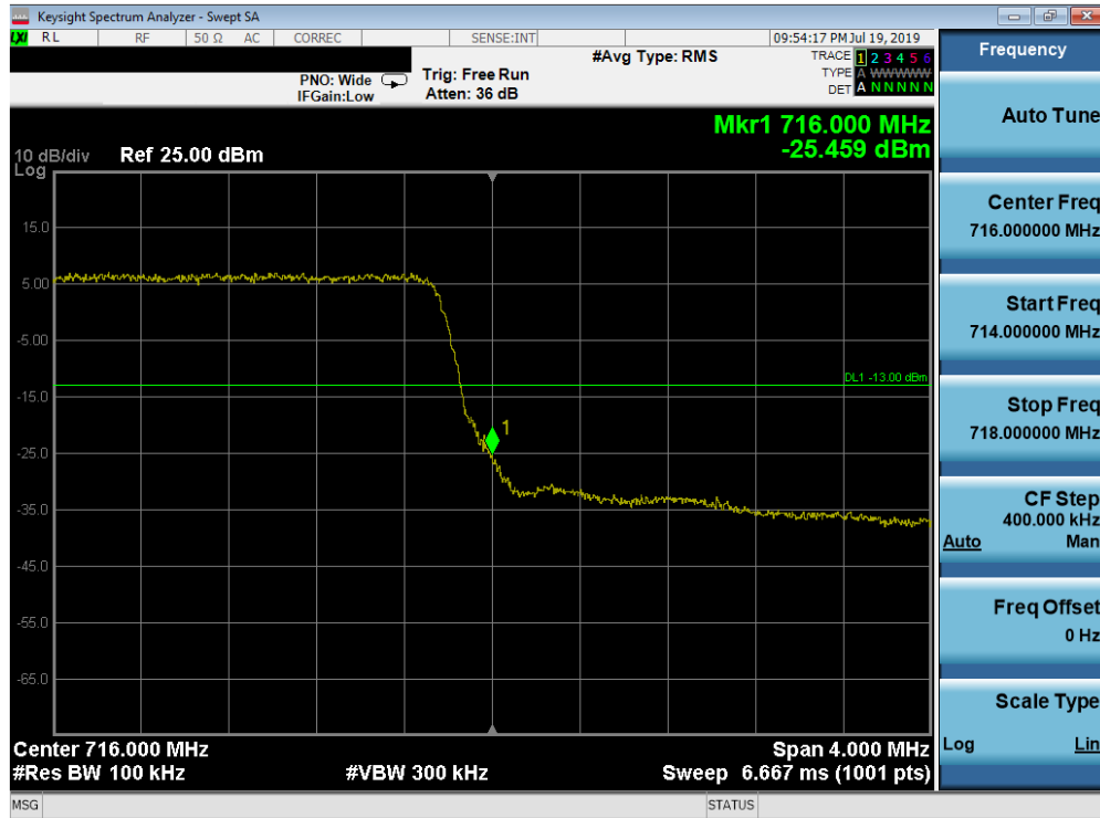
Plot 7-133. Upper Band Edge Plot (Band 12/17 - 5.0MHz QPSK - Full RB Configuration)
