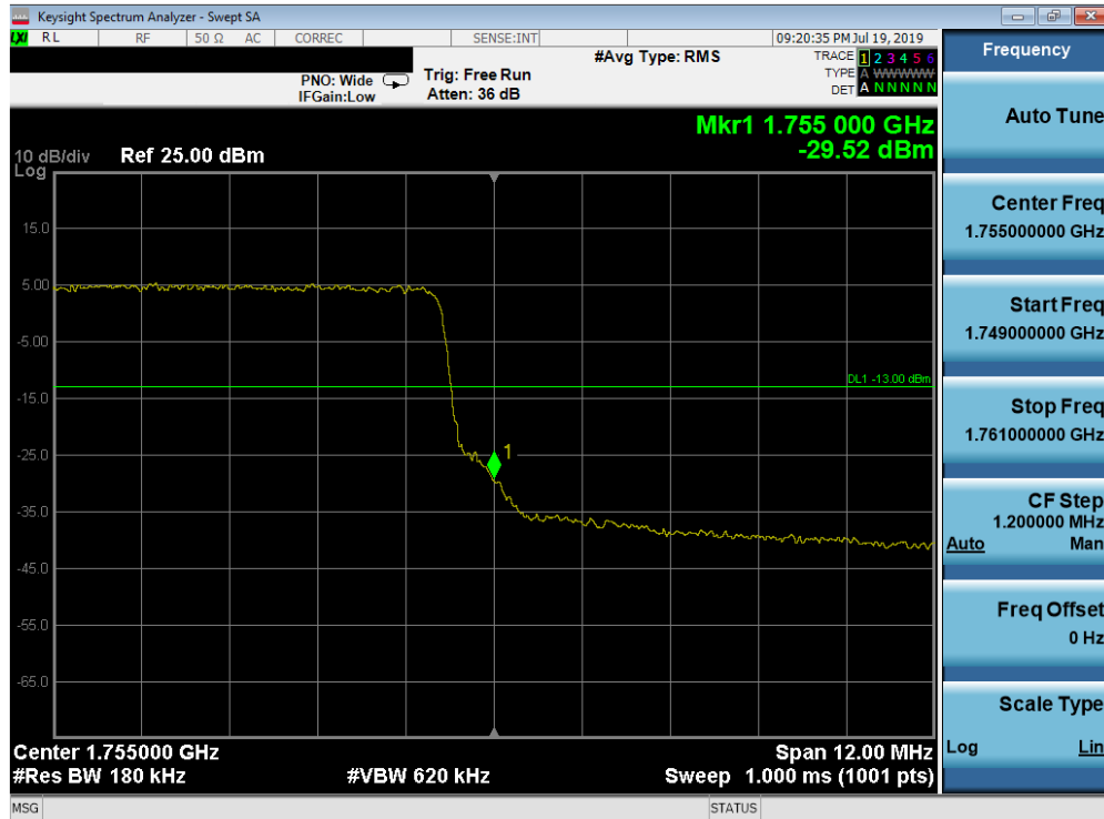
Plot 7-179. Upper Band Edge Plot (Band 4 - 15.0MHz QPSK - Full RB Configuration)
