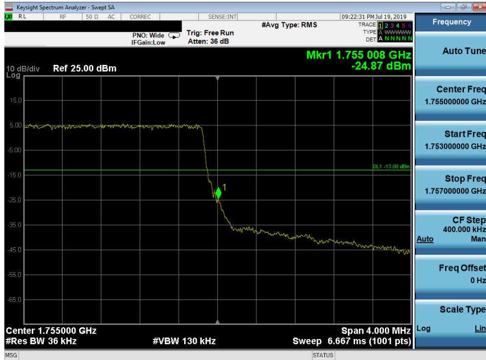
Plot 7-161. Upper Band Edge Plot (Band 4 - 3.0MHz QPSK - Full RB Configuration)
