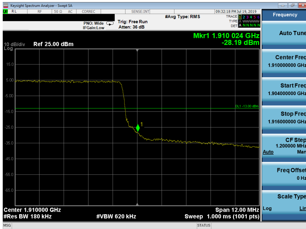
Plot 7-207. Upper Band Edge Plot (Band 2 - 15.0MHz QPSK - Full RB Configuration)
