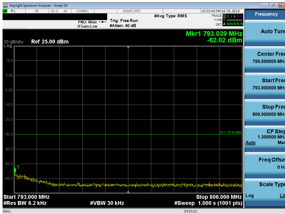
Plot 7-140. Upper Emission Mask Plot (Band 13 - 5.0MHz QPSK - Full RB Configuration)
