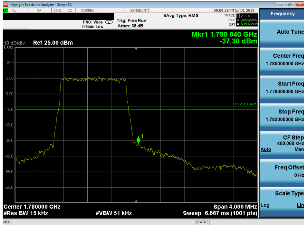
Plot 7-157. Upper Band Edge Plot (Band 66 - 1.4MHz QPSK - Full RB Configuration)
