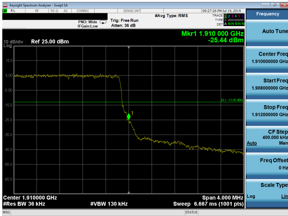
Plot 7-195. Upper Band Edge Plot (Band 2 - 3.0MHz QPSK - Full RB Configuration)
