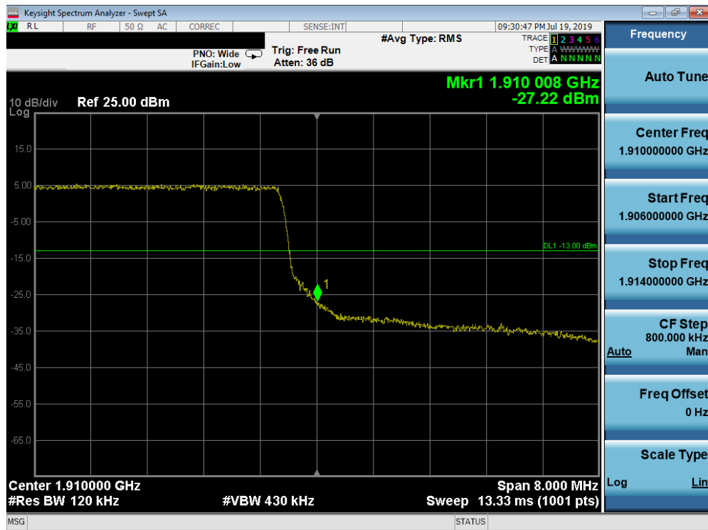
Plot 7-203. Upper Band Edge Plot (Band 2 - 10.0MHz QPSK - Full RB Configuration)
