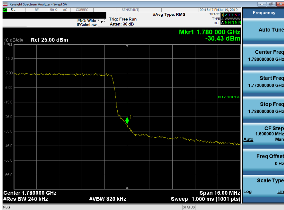
Plot 7-187. Upper Band Edge Plot (Band 66 - 20.0MHz QPSK - Full RB Configuration)
