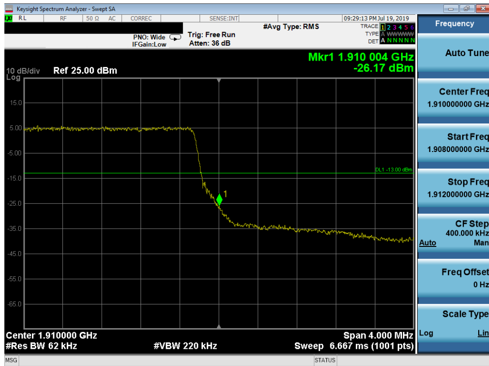
Plot 7-199. Upper Band Edge Plot (Band 2 - 5.0MHz QPSK - Full RB Configuration)
