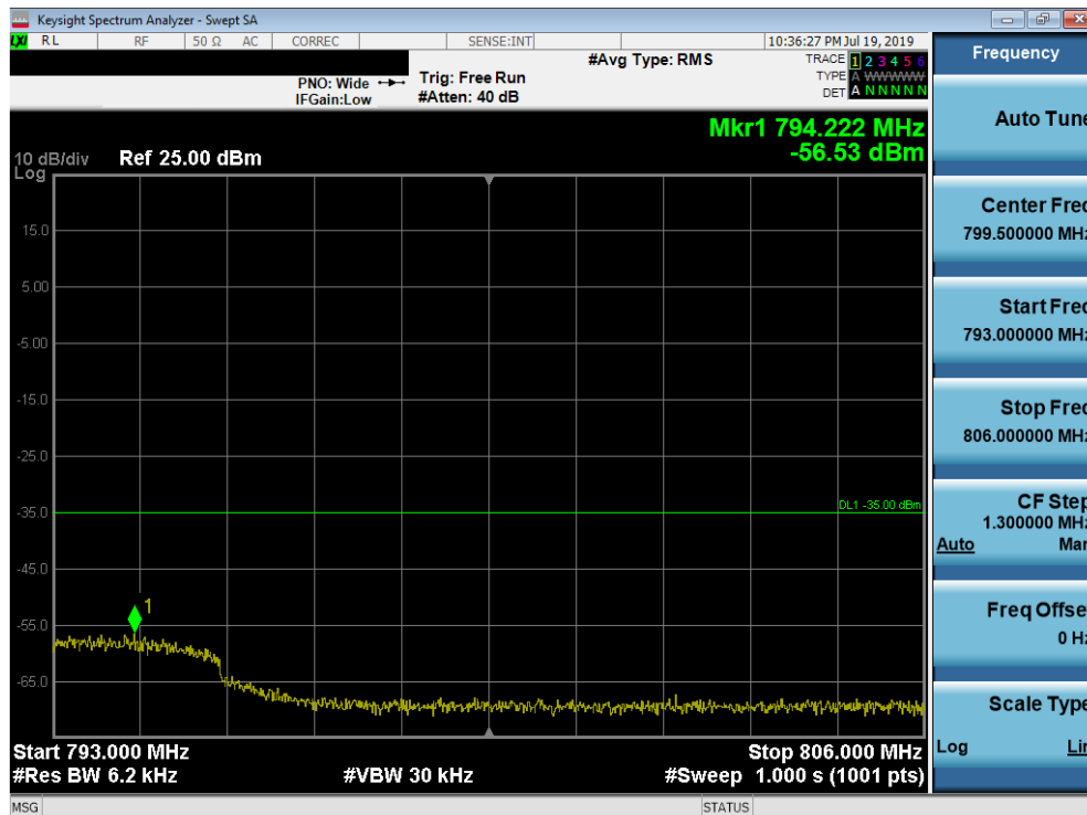
Plot 7-144. Upper Emission Mask Plot (Band 13 - 10.0MHz QPSK - Full RB Configuration)
