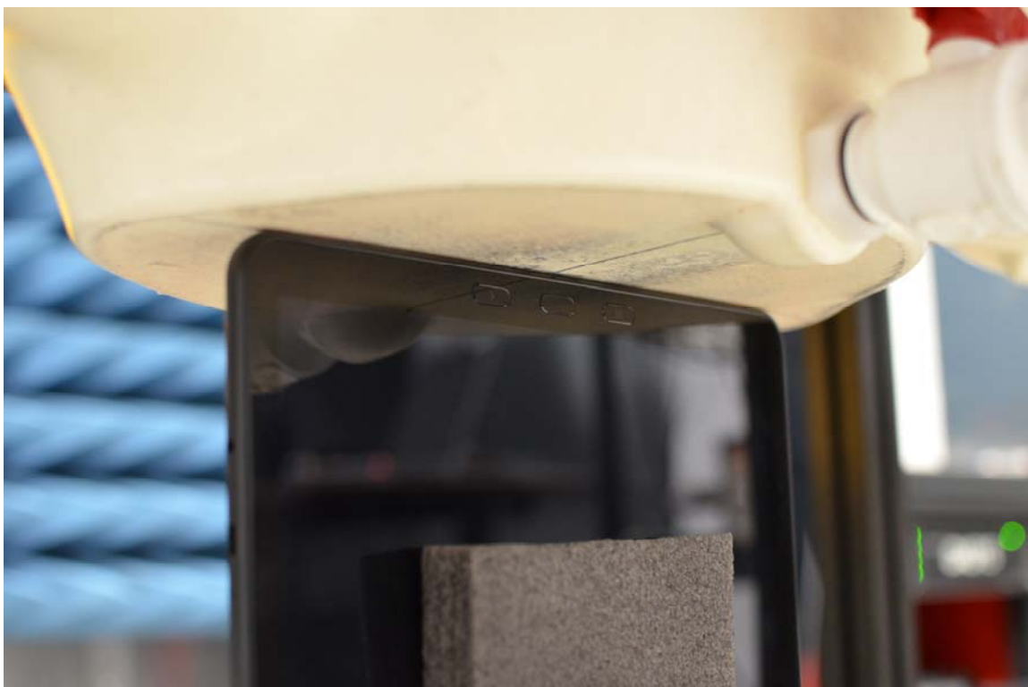
SAR Test Setup Photo 9 – Bottom Edge at 0 cm
