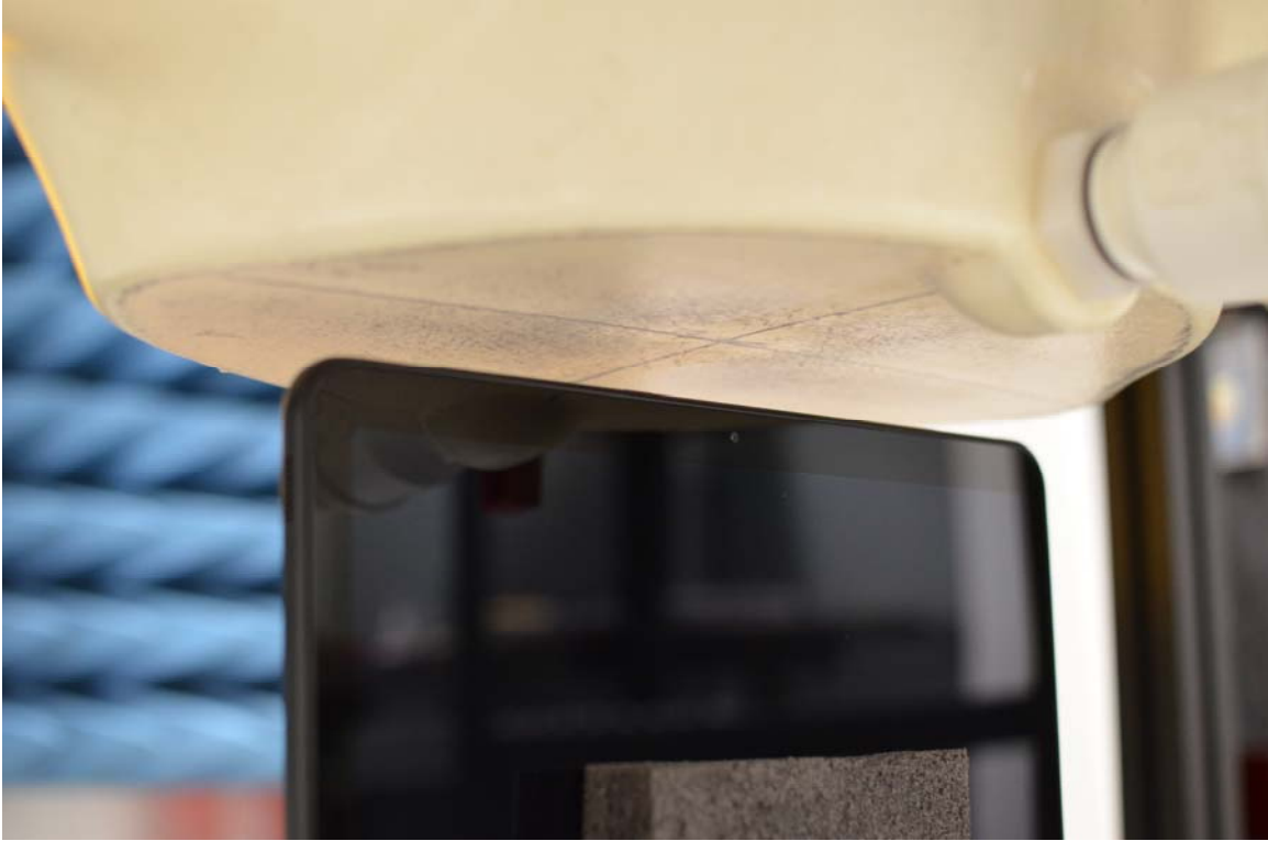
SAR Test Setup Photo 4 – Top Edge at 1.5 cm
