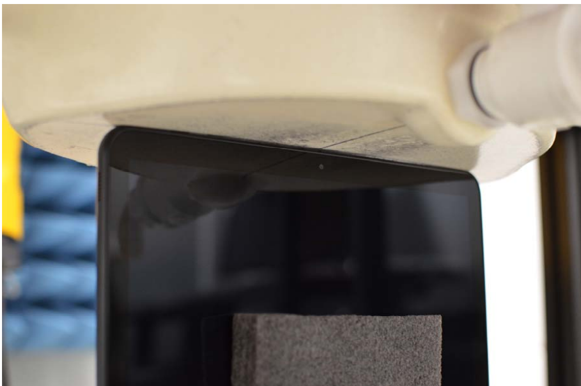
SAR Test Setup Photo 6 – Top Edge at 0 cm
