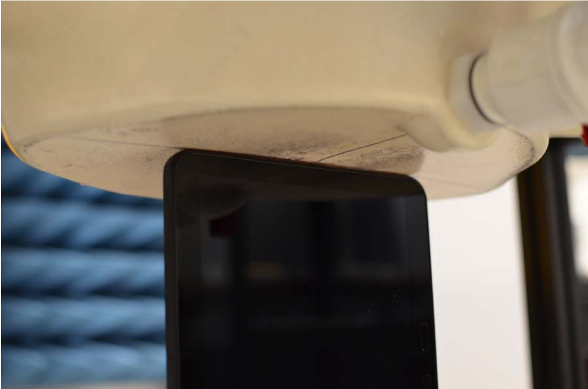
SAR Test Setup Photo 7 – Right Edge at 0 cm
