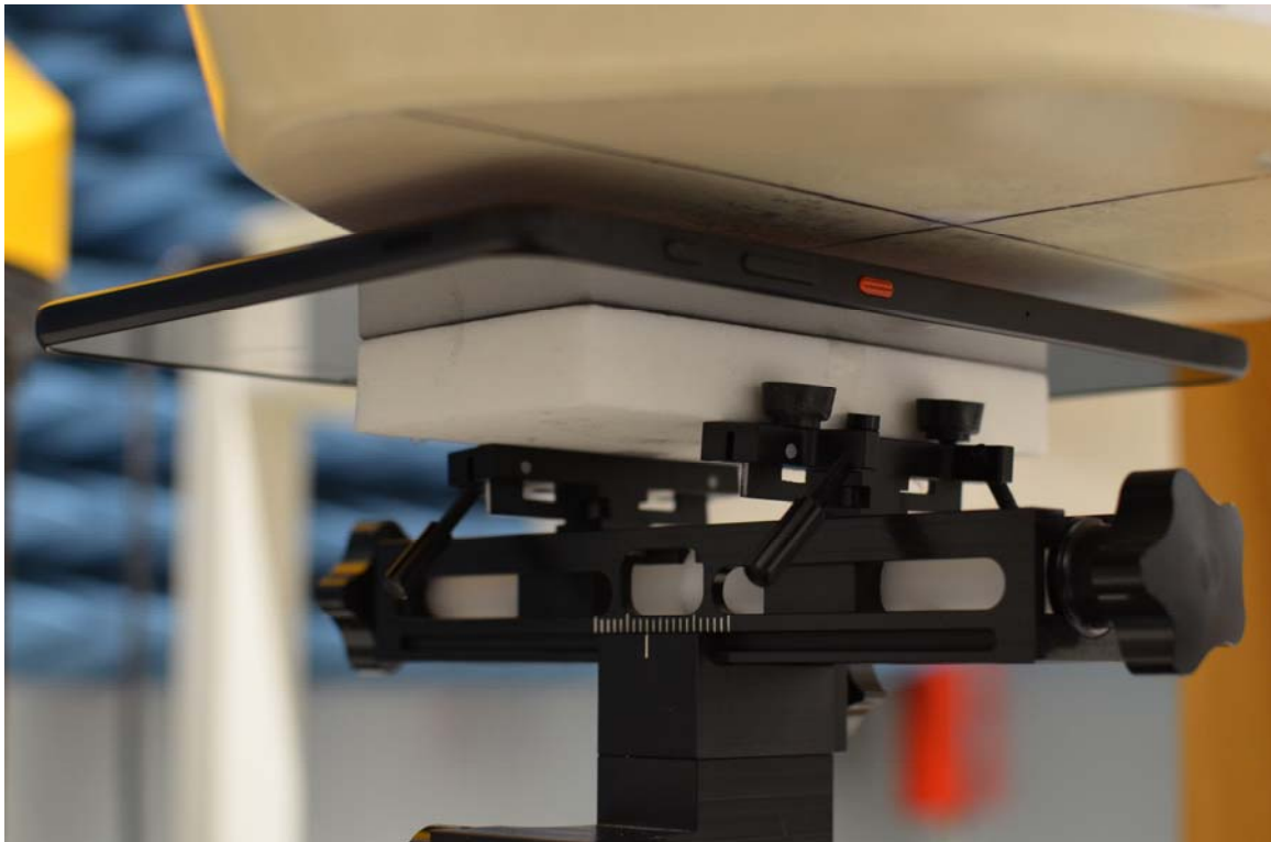
SAR Test Setup Photo 1 – Back Side at 1.0 cm
