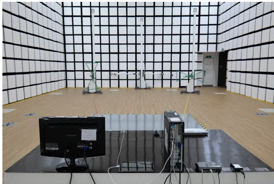
[ Radiated Disturbance for Below 1 GHz – Rear ]
