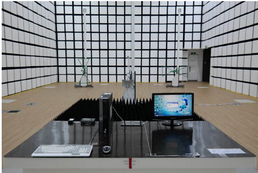
[ Radiated Disturbance for Above 1 GHz – Front ]
