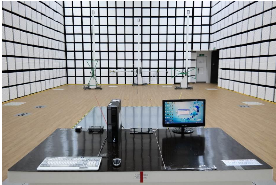
[ Radiated Disturbance for Below 1 GHz – Front ]
