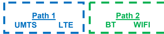
Figure 1-1 Simultaneous Transmission Paths
