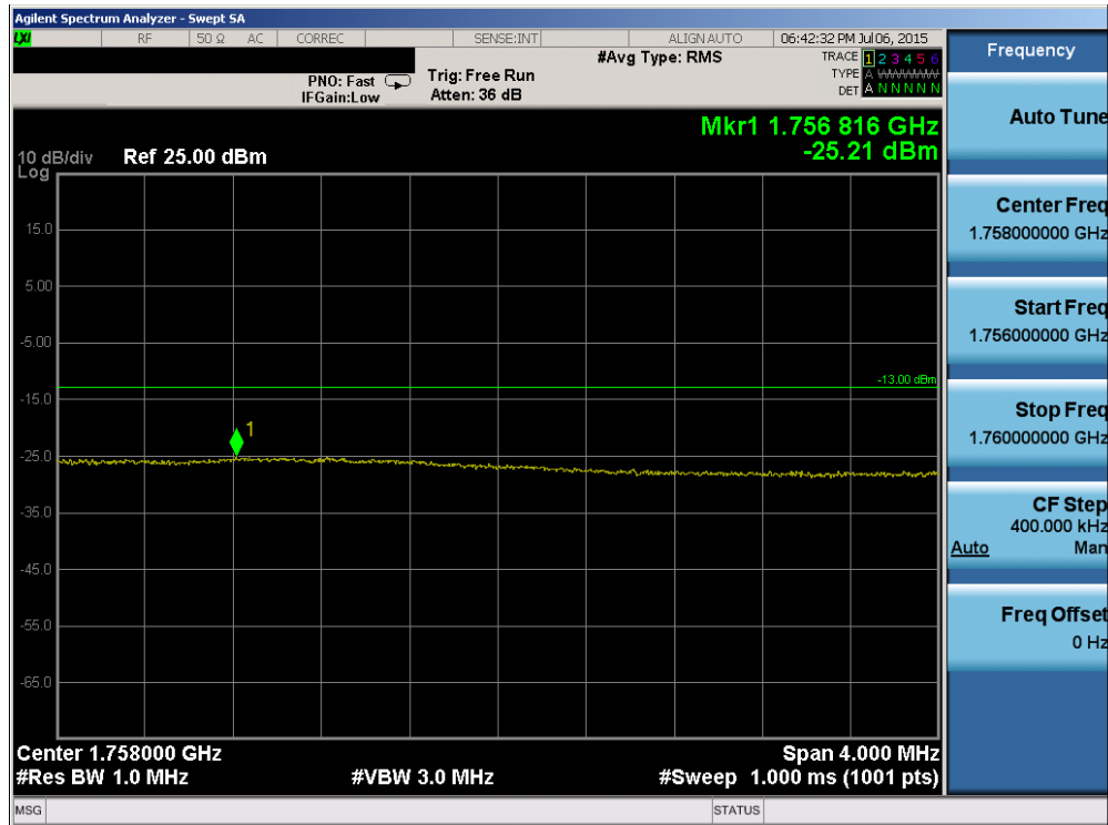
Plot 6-83. Upper Extended Band Edge Plot (Band 4 – 15.0MHz QPSK – RB Size 75)
