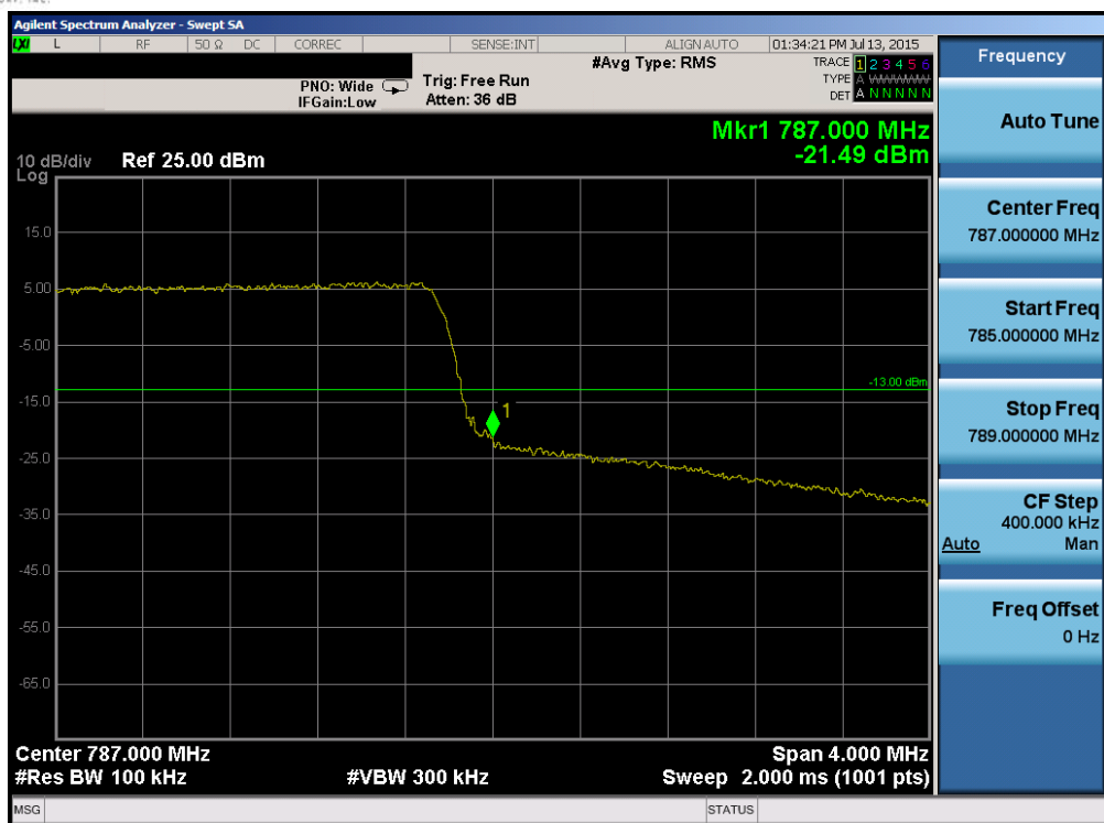
Plot 6-58. Upper Band Edge Plot (Band 13 - 5.0MHz QPSK - RB Size 25)
