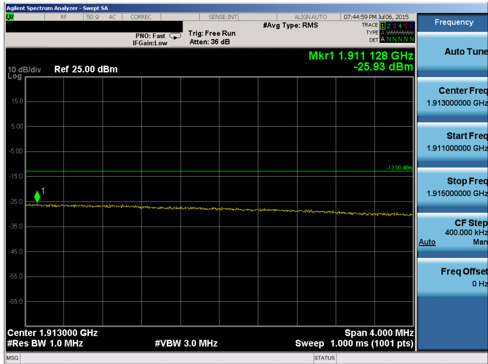
Plot 6-111. Upper Extended Band Edge Plot (Band 2 - 20.0MHz QPSK - RB Size 100)
