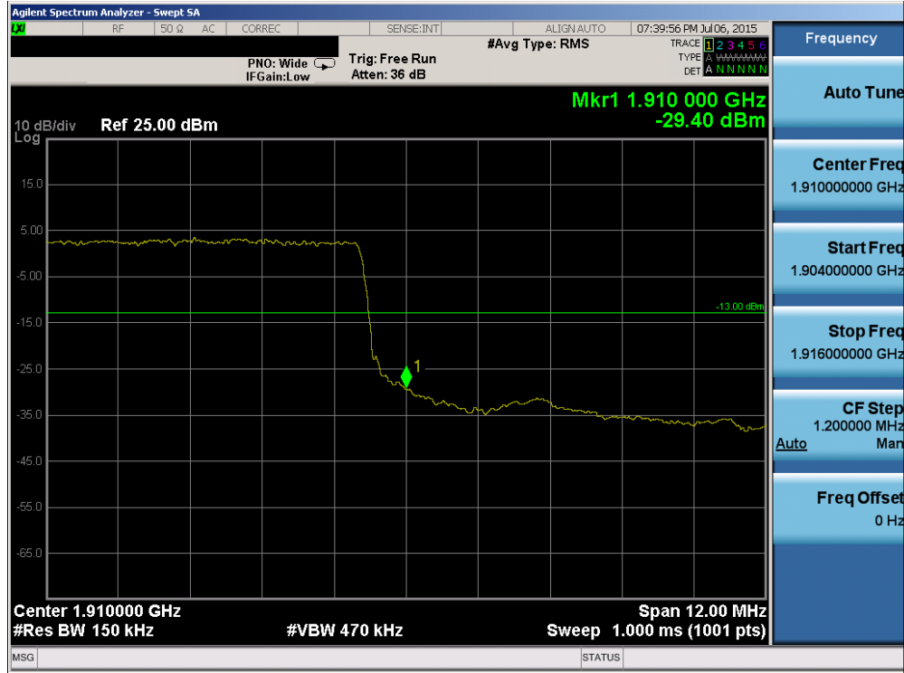
Plot 6-106. Upper Band Edge Plot (Band 2 – 15.0MHz QPSK – RB Size 75)
