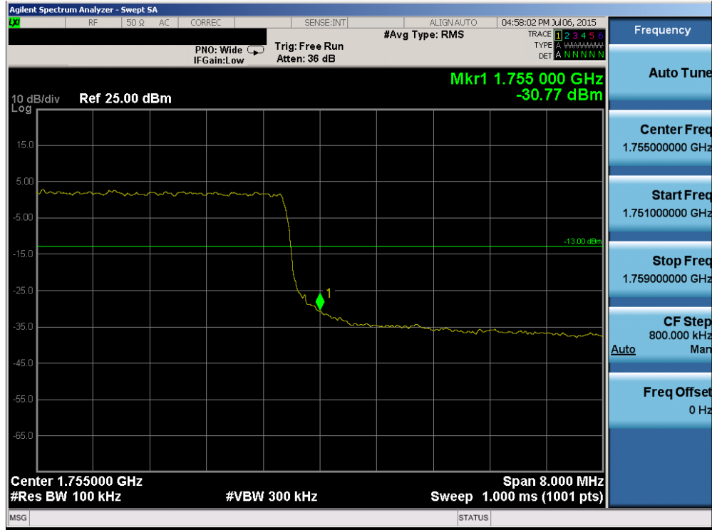
Plot 6-78. Upper Band Edge Plot (Band 4 – 10.0MHz QPSK – RB Size 50)
