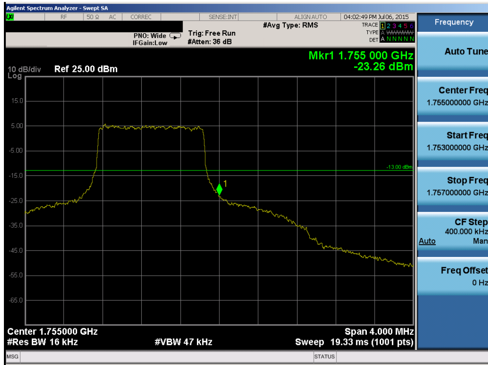
Plot 6-66. Upper Band Edge Plot (Band 4 – 1.4MHz QPSK – RB Size 6)
