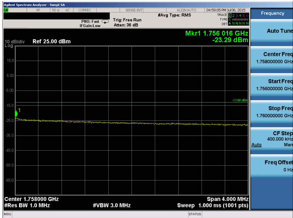
Plot 6-79. Upper Extended Band Edge Plot (Band 4 – 10.0MHz QPSK – RB Size 50)
