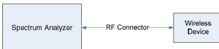
Figure 6-1. Test Instrument & Measurement Setup
