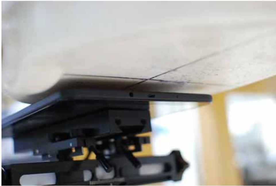
SAR Test Setup Photo 1: Back Side at 0.7 cm
