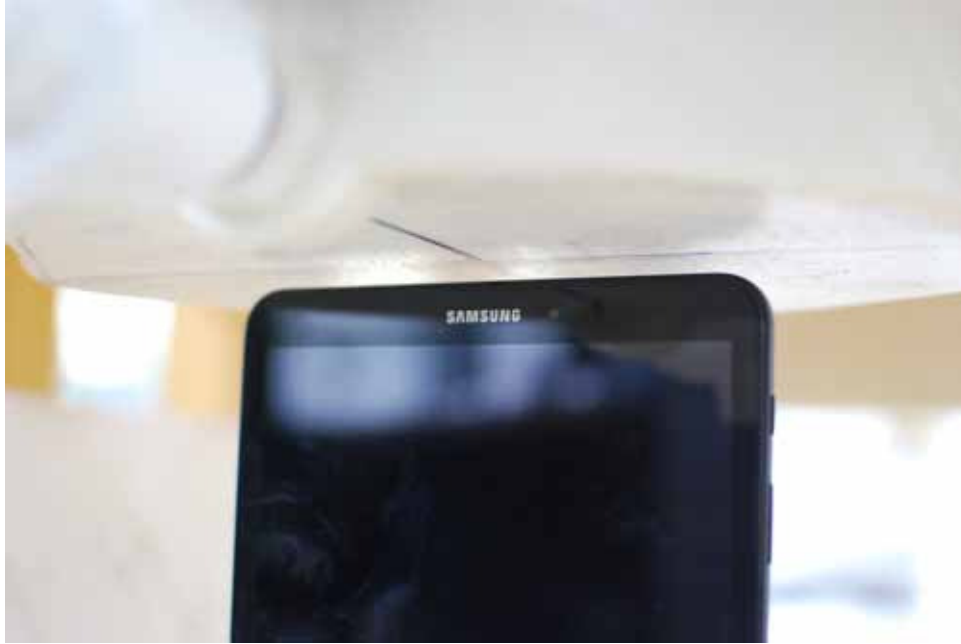
SAR Test Setup Photo 3: Top Edge at 0.4 cm
