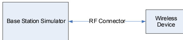
Figure 8-1 Power Measurement Setup
