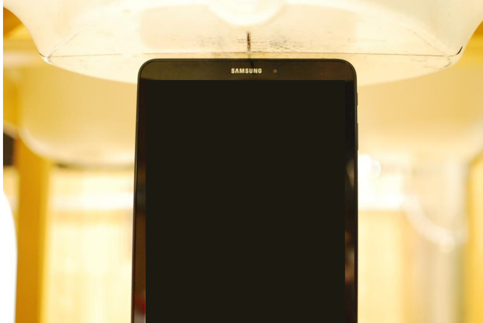
SAR Test Setup Photo 5: Top Edge at 0.4 cm
