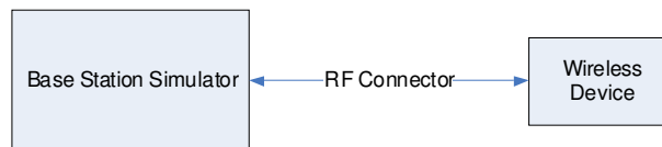
Figure 8-1 Power Measurement Setup
