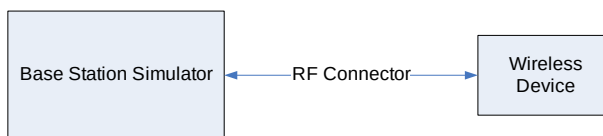
Figure 8-1 Power Measurement Setup
