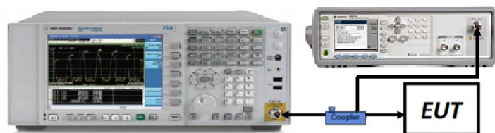
Figure 7-6. Test Instrument & Measurement Setup
