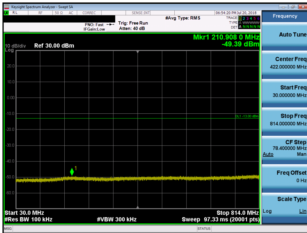
Plot 7-15. Conducted Spurious Plot (CDMA, Ch. 684)
