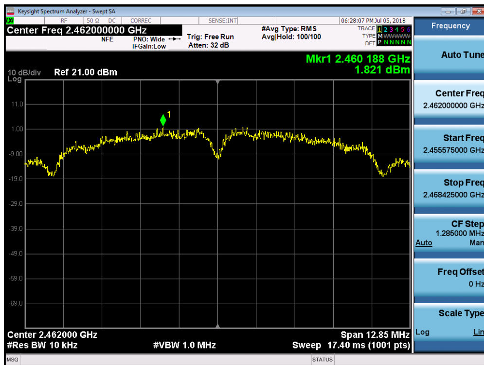
Plot 7-12. Power Spectral Density Plot (802.11b – Ch. 11)
