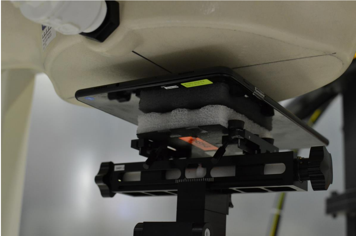
SAR Test Setup Photo 1 – Back Side at 2.2 cm
