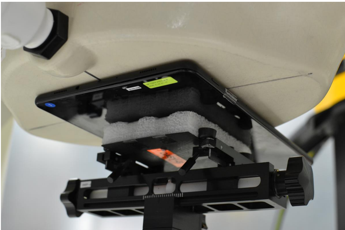
SAR Test Setup Photo 4 – Back Side at 0.0 cm
