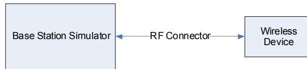
Figure 8-1 Power Measurement Setup
