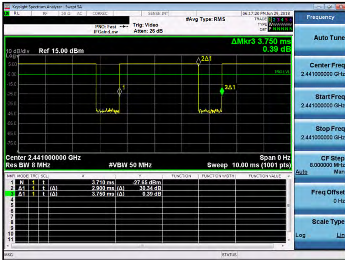
Figure 8-3 Bluetooth Transmission Plot
