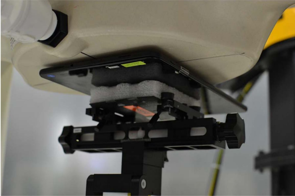
SAR Test Setup Photo 3 – Back Side at 0.7 cm
