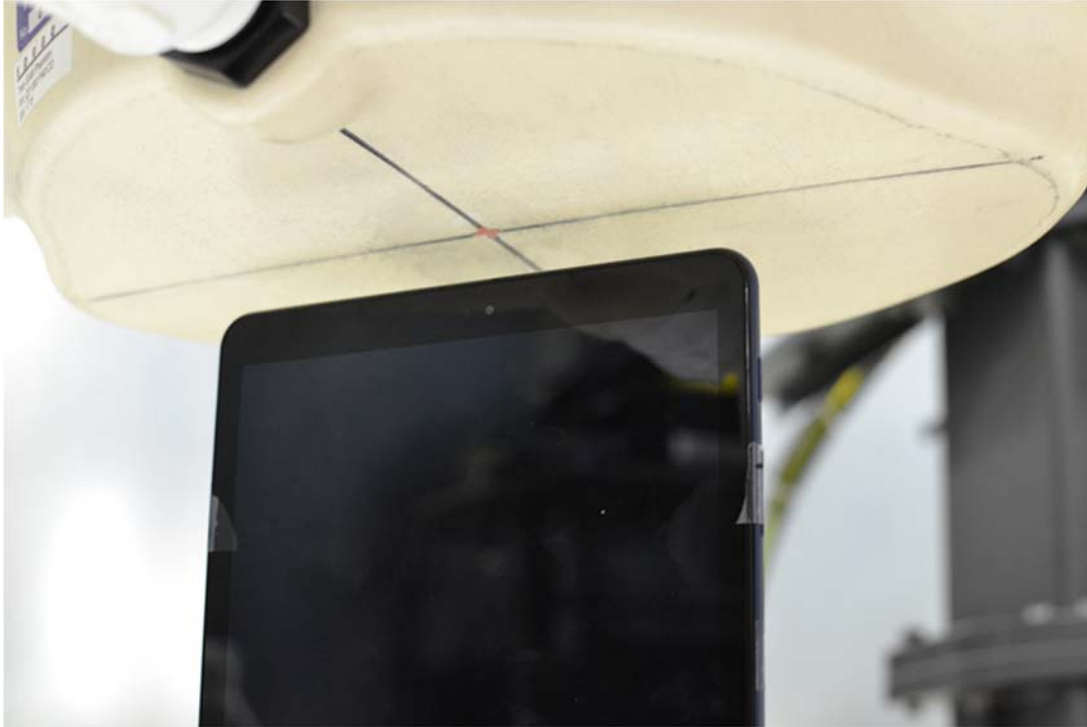
SAR Test Setup Photo 5 – Top Edge at 1.7 cm
