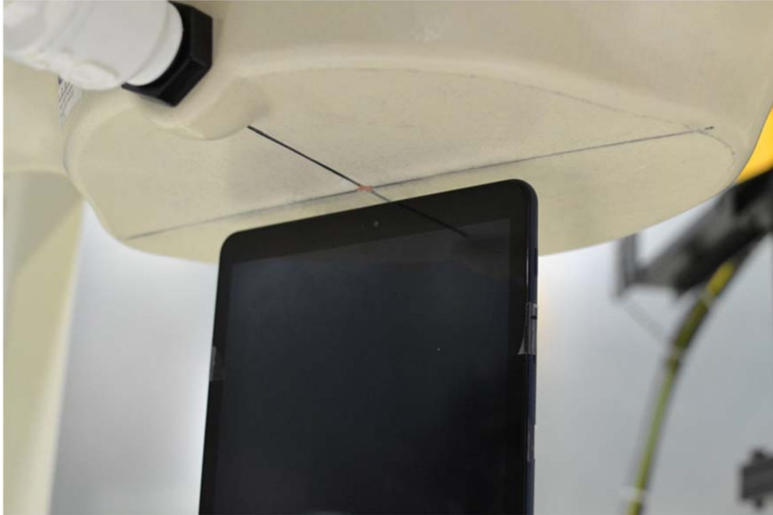
SAR Test Setup Photo 7 – Top Edge at 0.7 cm
