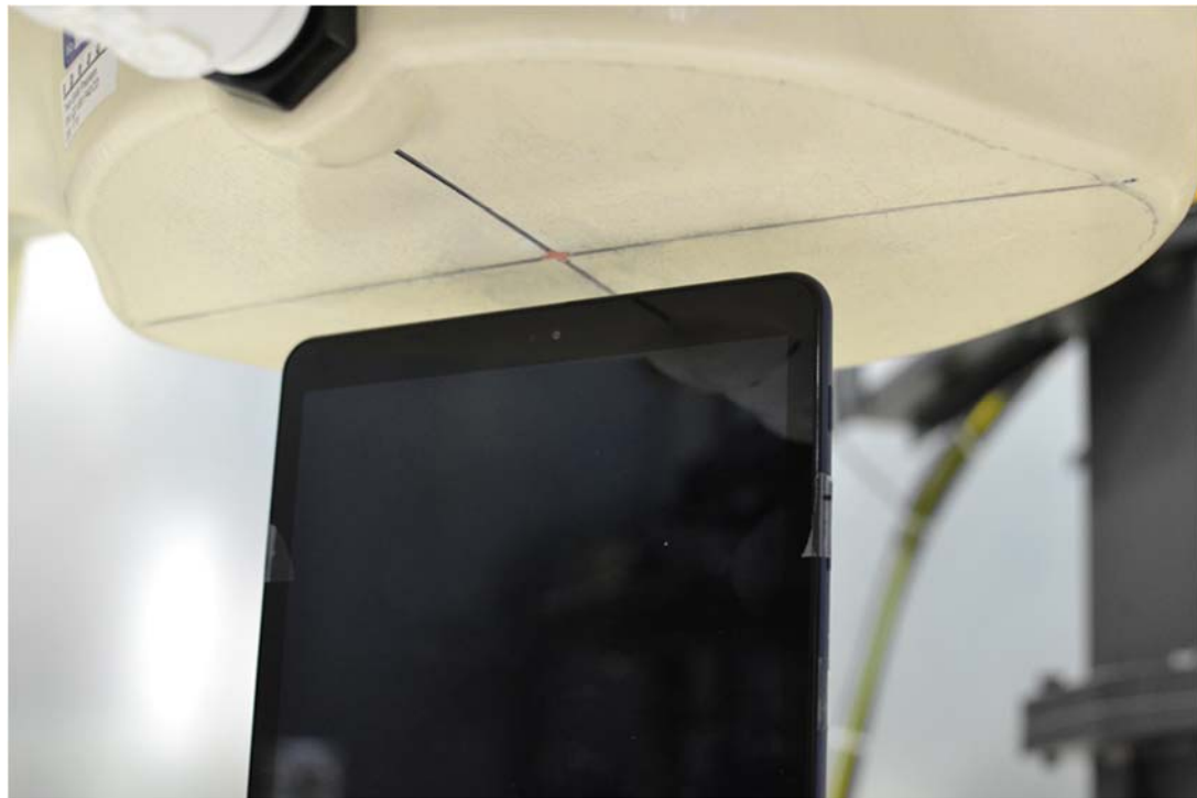
SAR Test Setup Photo 6 – Top Edge at 1.4 cm
