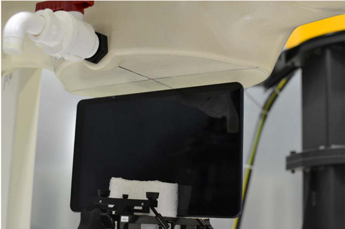
SAR Test Setup Photo 9 – Right Edge at 1.4 cm
