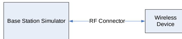
Figure 9-3 Power Measurement Setup
