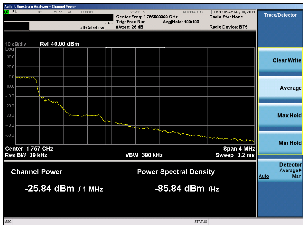
Plot 6-172. Upper Extended Band Edge Plot (Band 4 – 1.4MHz QPSK – RB Size 6)
