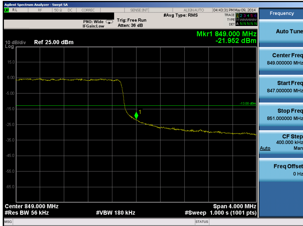
Plot 6-163. Upper Band Edge Plot (Band 5 - 5.0MHz QPSK - RB Size 25)
