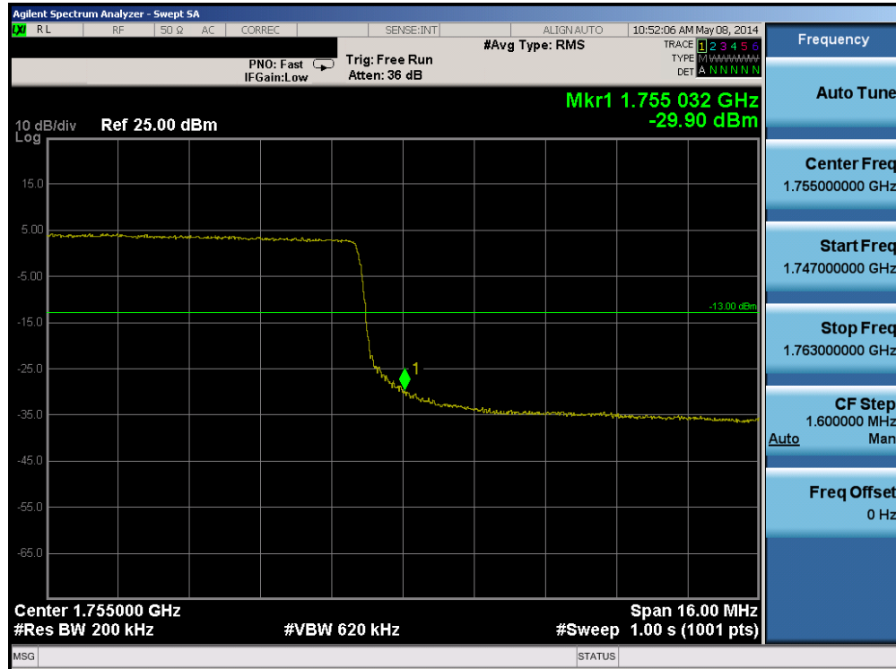
Plot 6-191. Upper Band Edge Plot (Band 4 – 20.0MHz QPSK – RB Size 100)
