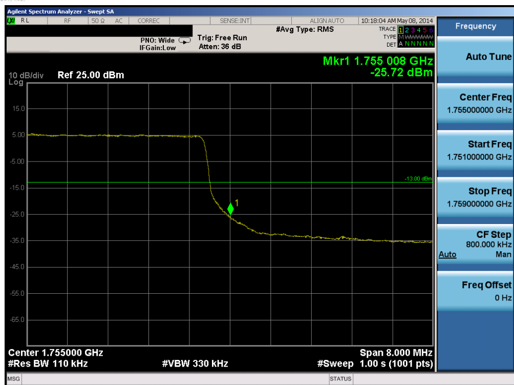
Plot 6-183. Upper Band Edge Plot (Band 4 – 10.0MHz QPSK – RB Size 50)
