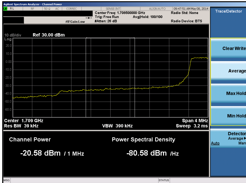
Plot 6-174. Lower Extended Band Edge Plot (Band 4 – 3.0MHz QPSK – RB Size 15)
