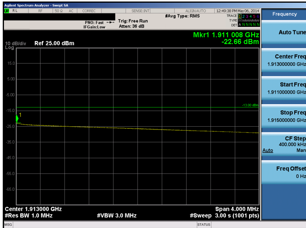
Plot 6-208. Upper Extended Band Edge Plot (Band 2 - 10.0MHz QPSK - RB Size 50)
