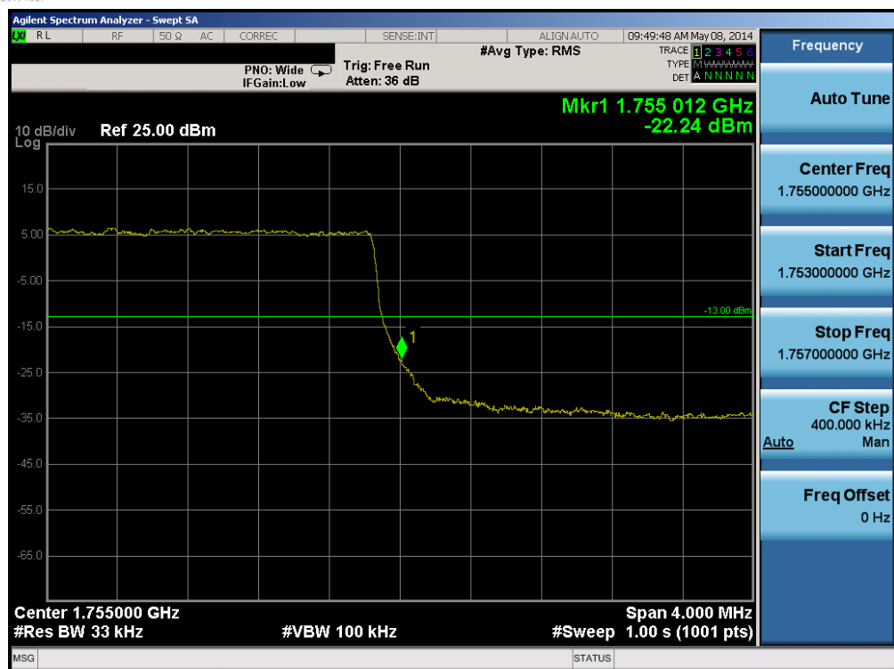
Plot 6-175. Upper Band Edge Plot (Band 4 – 3.0MHz QPSK – RB Size 15)
