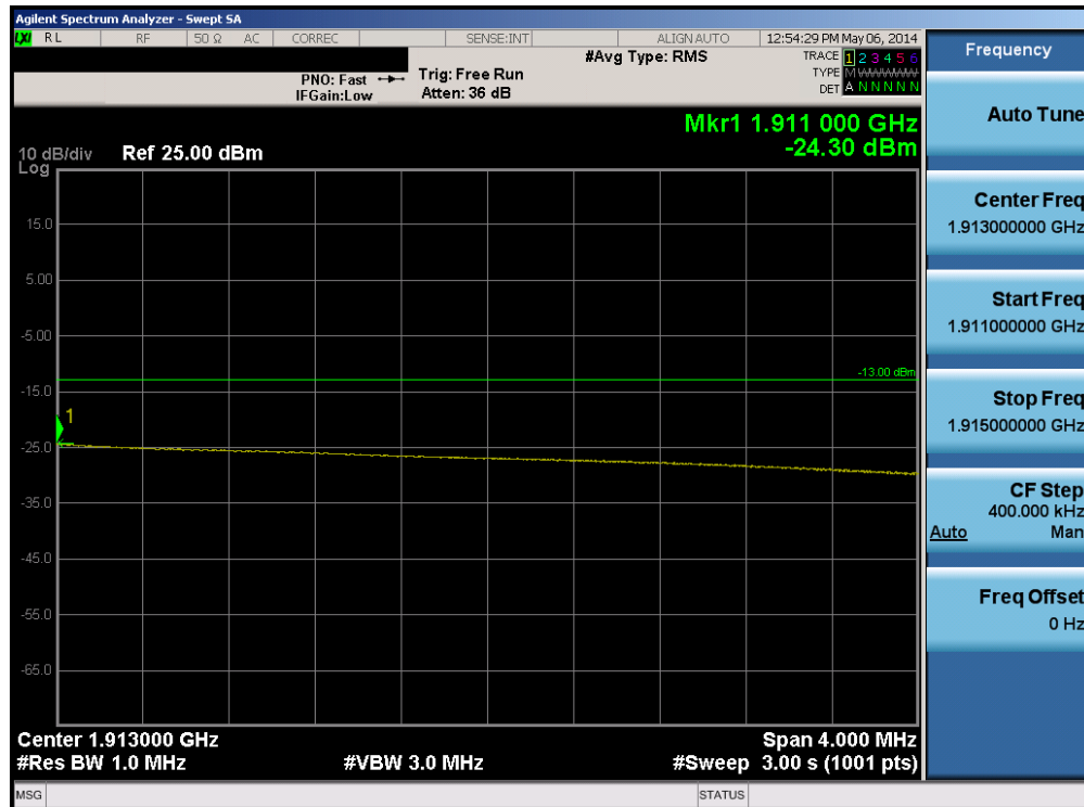
Plot 6-212. Upper Extended Band Edge Plot (Band 2 – 15.0MHz QPSK – RB Size 75)
