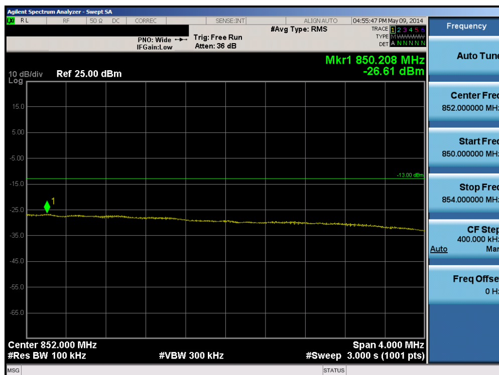
Plot 6-168. Upper Extended Band Edge Plot (Band 5 – 10.0MHz QPSK – RB Size 50)
