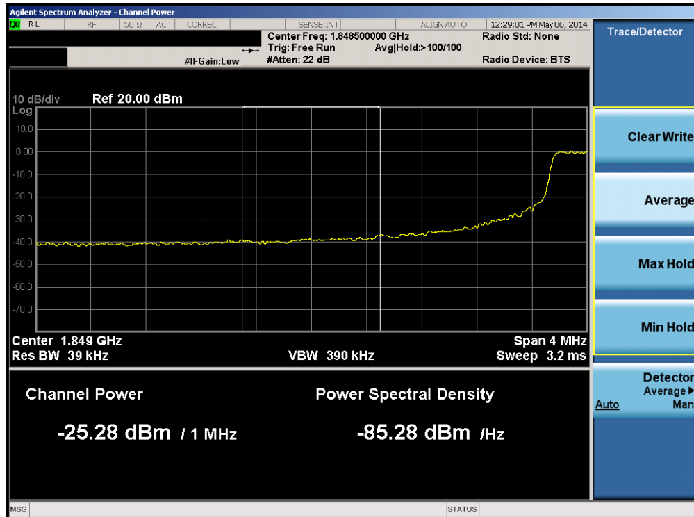
Plot 6-202. Lower Extended Band Edge Plot (Band 2 – 5.0MHz QPSK – RB Size 25)
