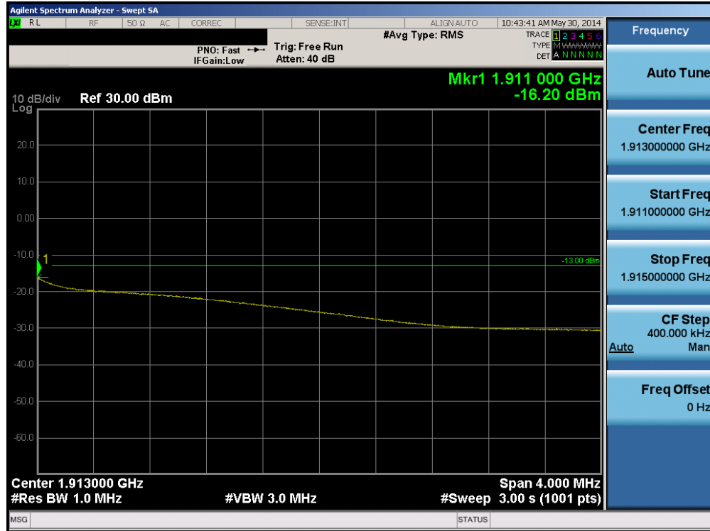
Plot 6-43. 4MHz Span Plot (PCS WCDMA Mode – Ch. 9538)
