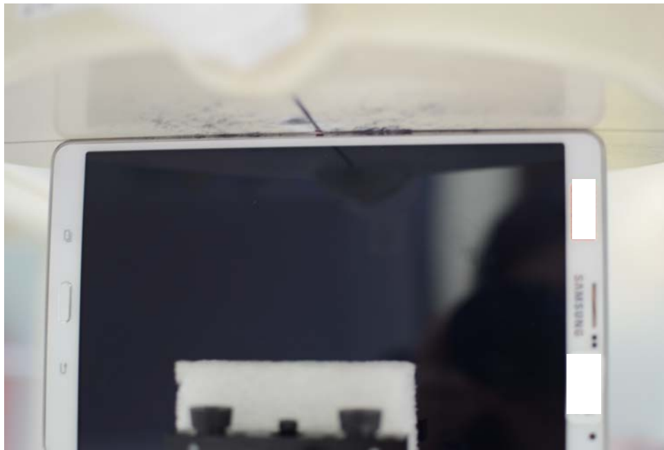
SAR Test Setup Photo 12 – Left Edge at 0 mm
