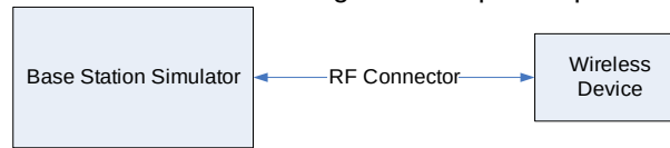
Figure 8-1 Power Measurement Setup
