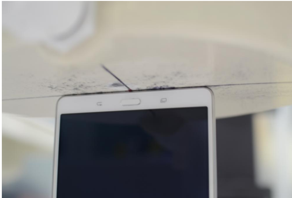
SAR Test Setup Photo 4 – Bottom Edge at 0.0 mm
