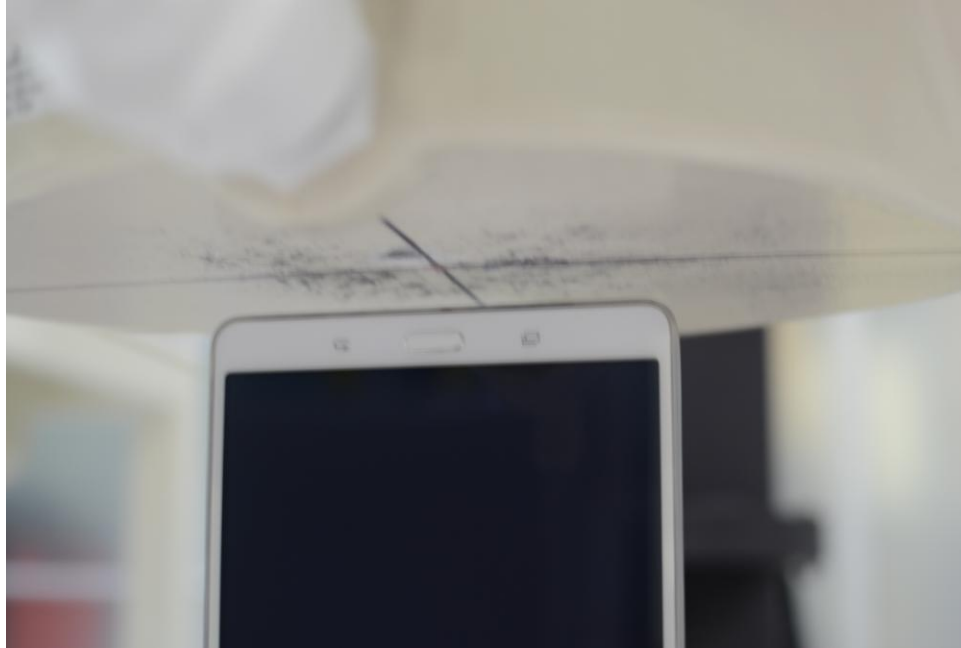
SAR Test Setup Photo 5 – Bottom Edge at 13 mm
