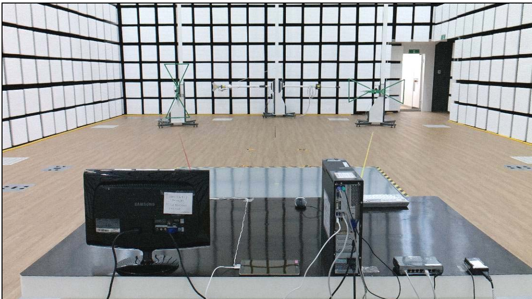
[ Radiated Disturbance for Below 1 GHz – Rear ]
