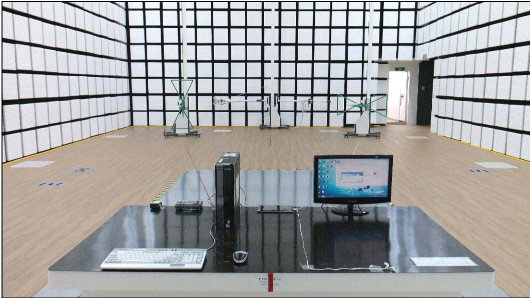
[ Radiated Disturbance for Below 1 GHz – Front ]
