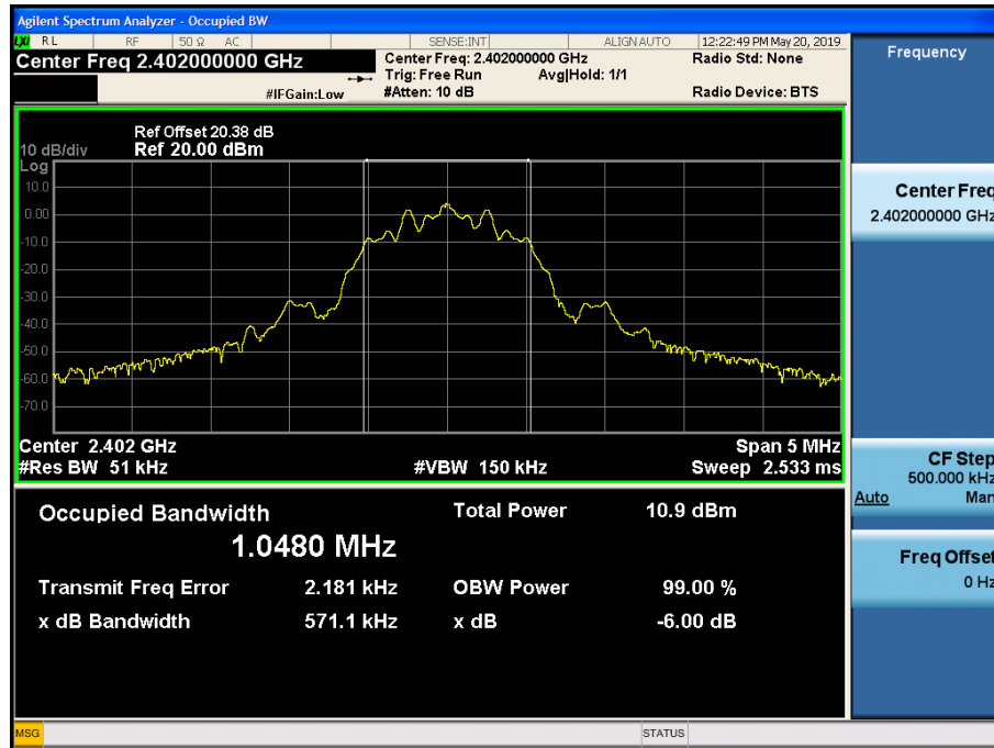
99 % Bandwidth plot (Low-CH 0)
