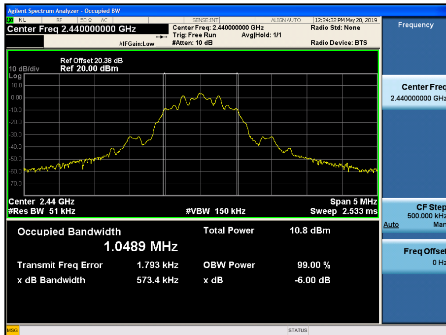
99 % Bandwidth plot (Mid-CH 19)
