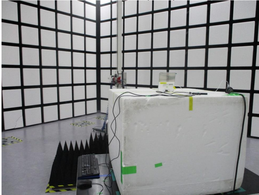
ABOVE 1 GHz REAR TEST PHOTO(X axis)
