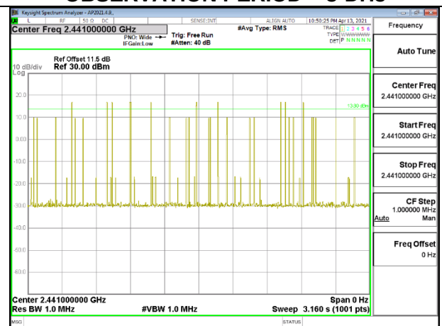
NUMBER OF PULSES IN 3.16 SECOND OBSERVATION PERIOD – 3-DH5
