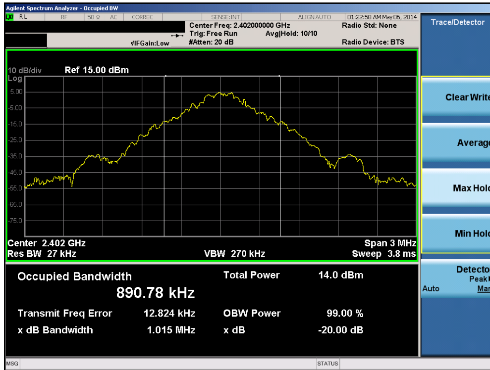
Plot 6-1. 20dB Bandwidth Plot (Bluetooth, 1Mbps – Ch. 0)
