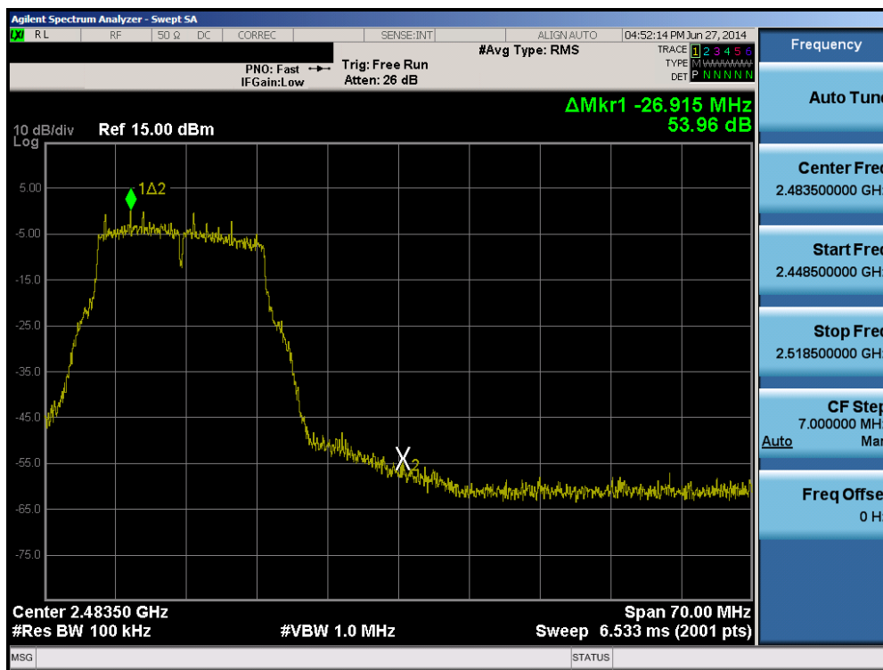
Plot 6-90. Band Edge Plot (802.11g - Ch. 11)
