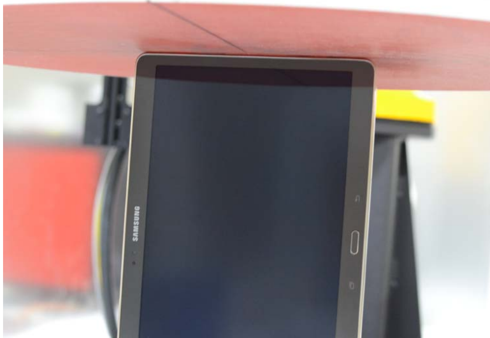
SAR Test Setup Photo 5 – Right Edge at 0 mm
