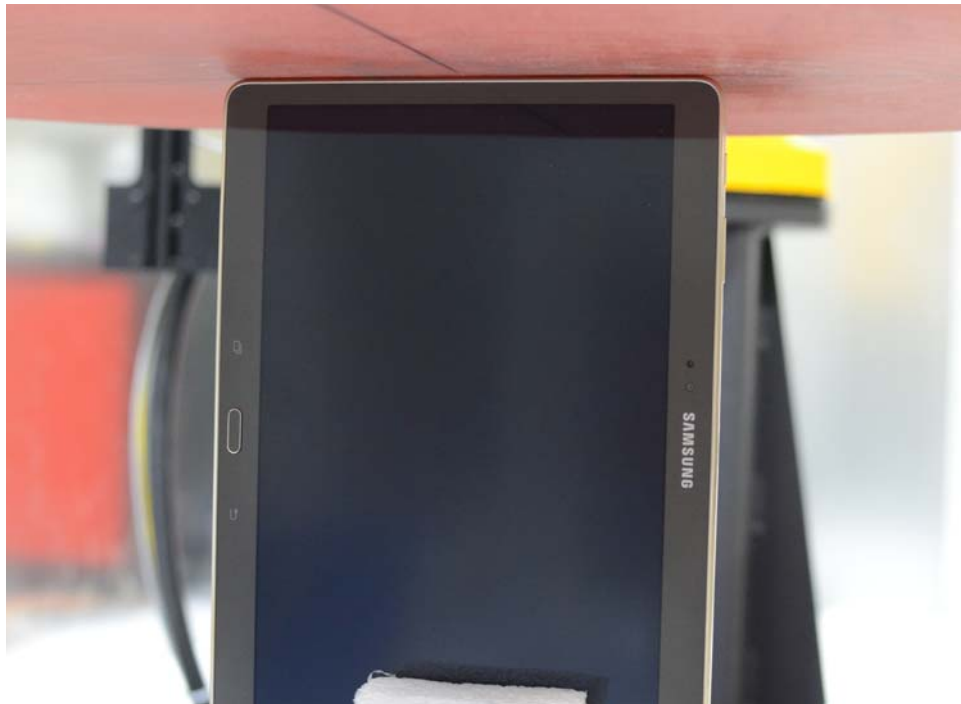
SAR Test Setup Photo 6 – Left Edge at 0 mm
