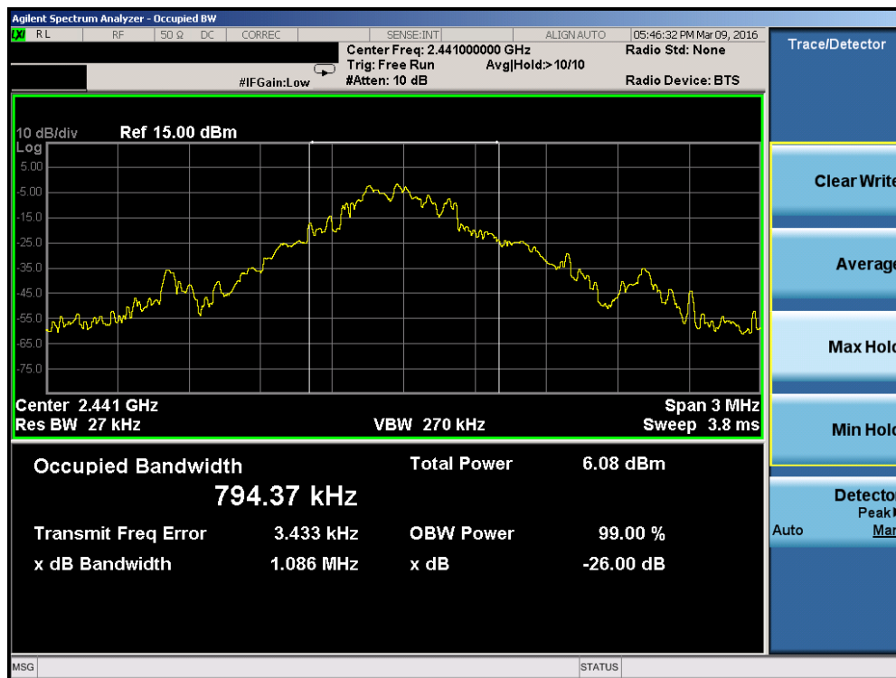
Plot 7-1. Occupied Bandwidth Plot (ANT+ – Ch. 39)
