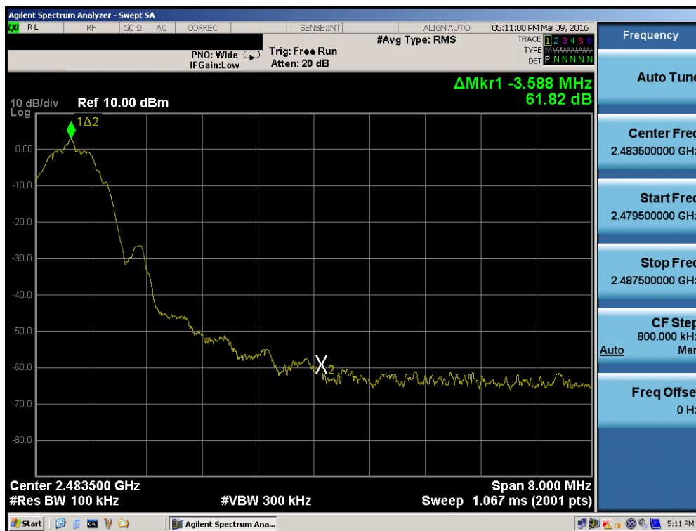
Plot 7-11. Band Edge Plot (Bluetooth (LE) – Ch. 39)
