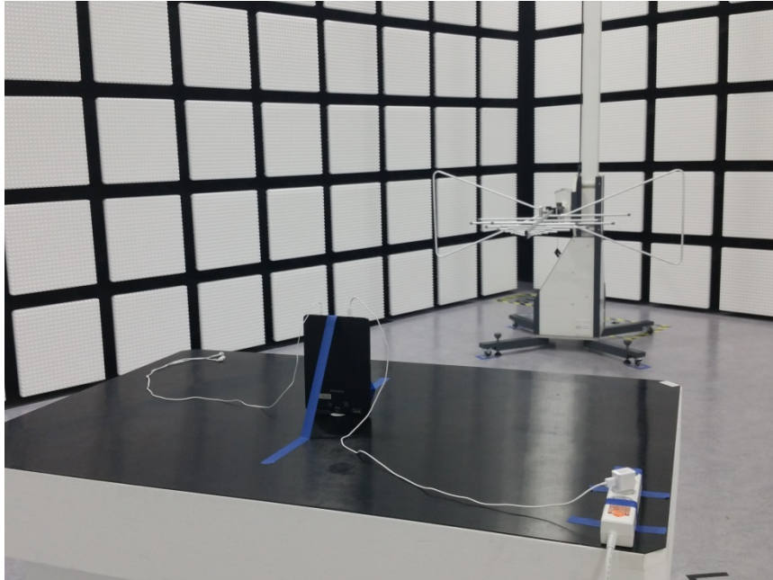
RADIATED BACK PHOTO (BELOW 1 GHz)
