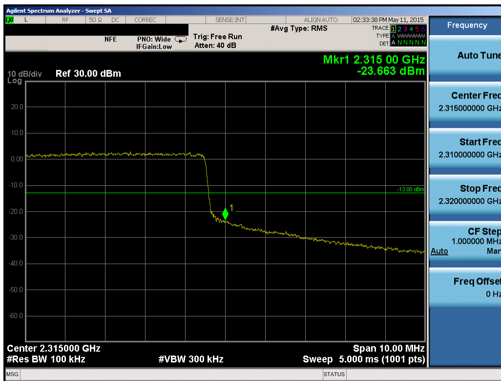
Plot 6-168. Upper Band Edge Plot (Band 30 – 10.0MHz QPSK – RB Size 50)
