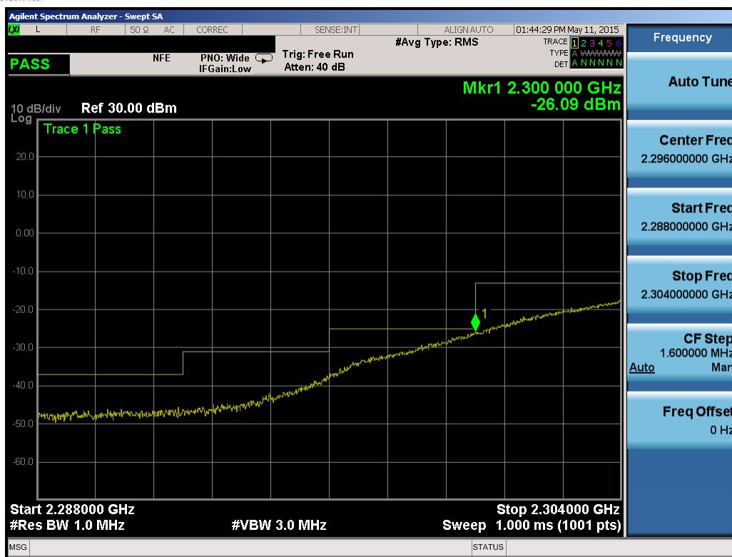
Plot 6-167. Lower Extended Band Edge Plot (Band 30 – 10.0MHz QPSK – RB Size 50)
