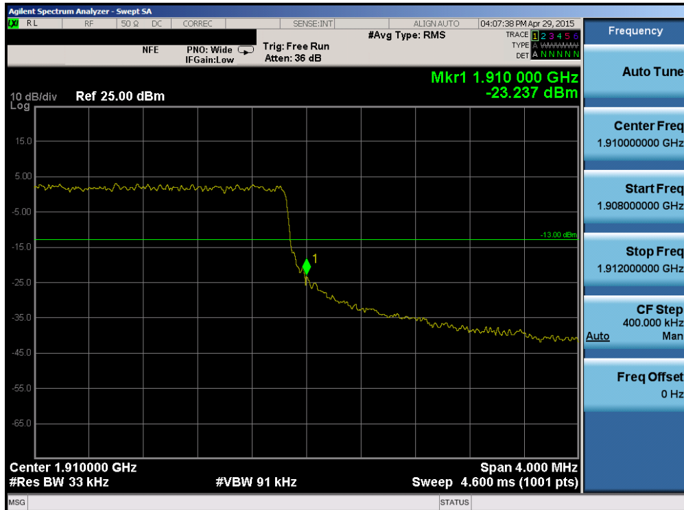
Plot 6-144. Upper Band Edge Plot (Band 2 – 3.0MHz QPSK – RB Size 15)
