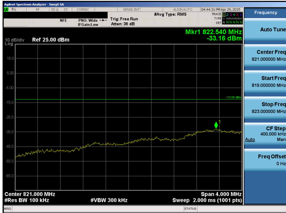
Plot 6-99. Lower Extended Band Edge Plot (Band 5 – 1.4MHz QPSK – RB Size 6)
