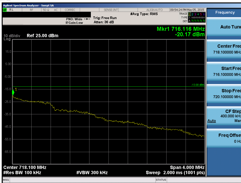
Plot 6-87. Upper Extended Band Edge Plot (Band 12 – 1.4MHz QPSK – RB Size 6)
