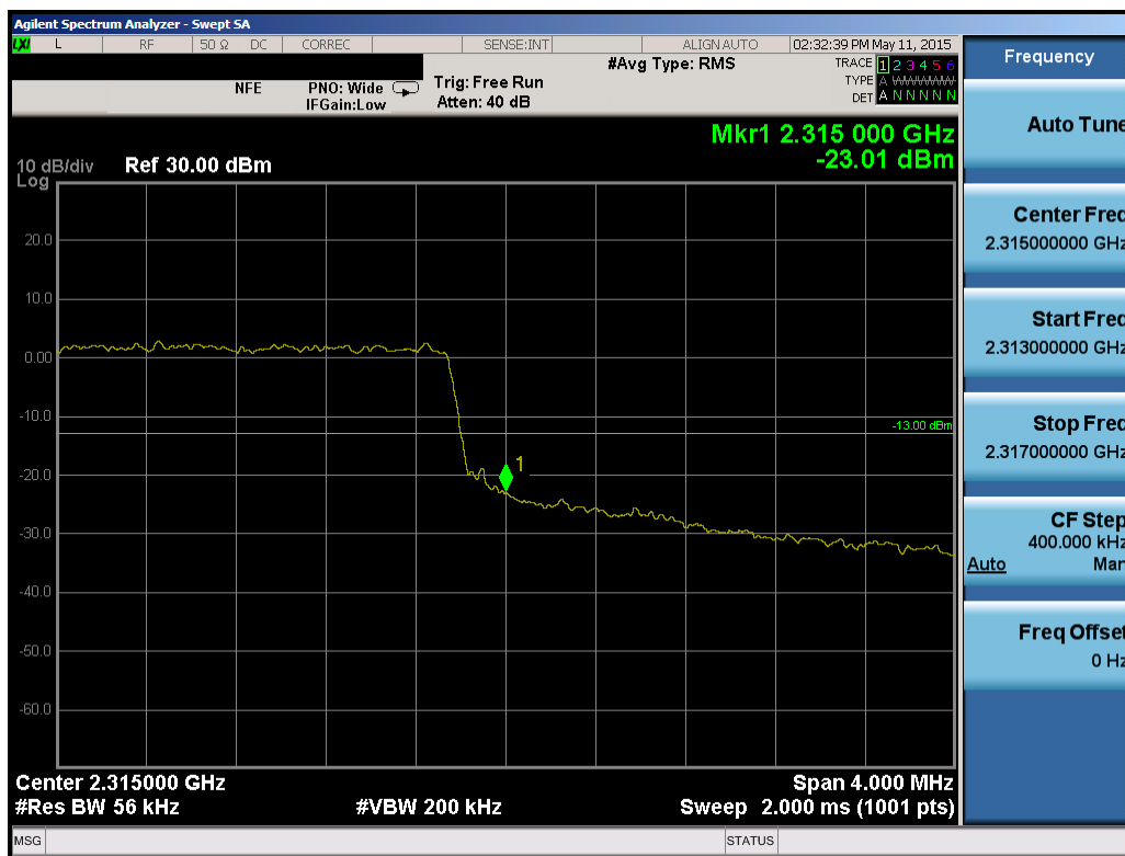
Plot 6-164. Upper Band Edge Plot (Band 30 – 5.0MHz QPSK – RB Size 25)
