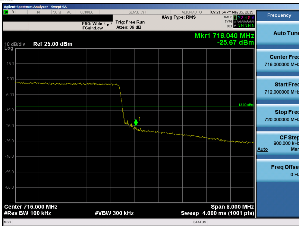
Plot 6-97. Upper Band Edge Plot (Band 12 – 10.0MHz QPSK – RB Size 50)
