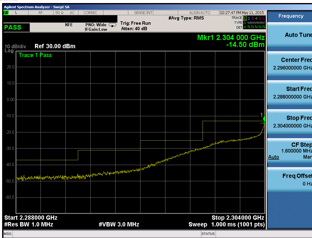
Plot 6-163. Lower Extended Band Edge Plot (Band 30 – 5.0MHz QPSK – RB Size 25)
