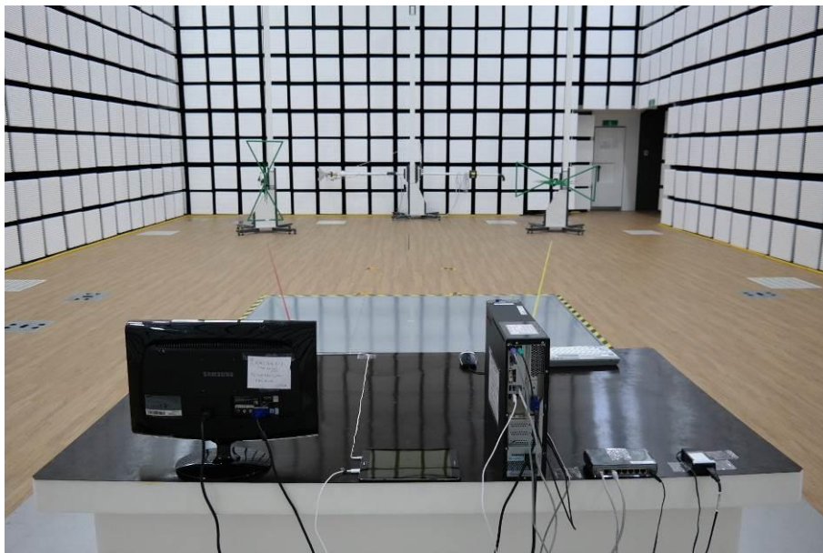
[ Radiated Disturbance for Below 1 GHz – Rear ]
