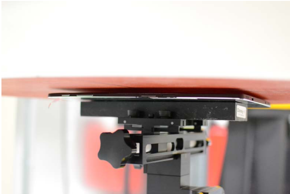
SAR Test Setup Photo 2: Back Side at 0.4 cm
