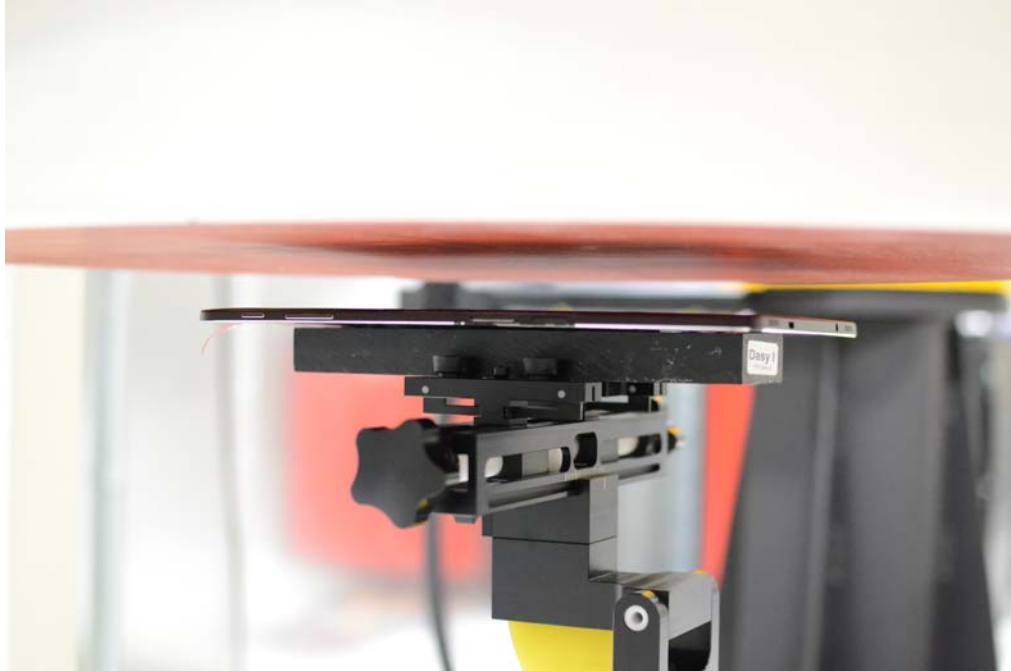
SAR Test Setup Photo 3: Back Side at 2.4 cm
