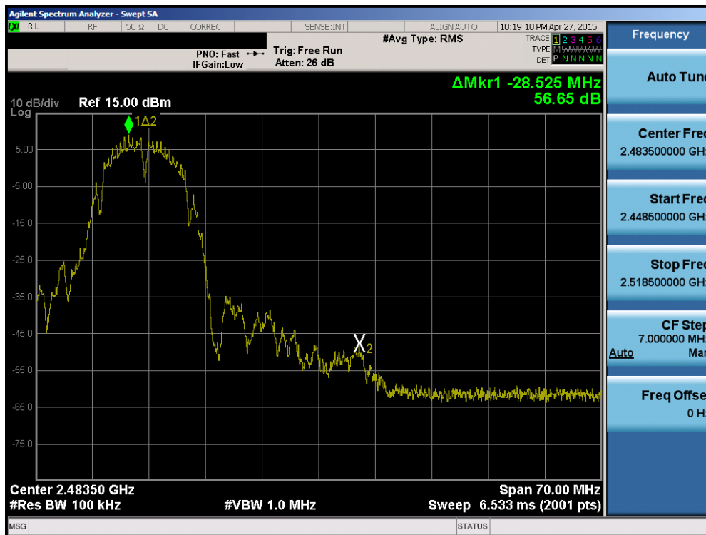
Plot 6-44. Band Edge Plot (802.11b – Ch. 11)
