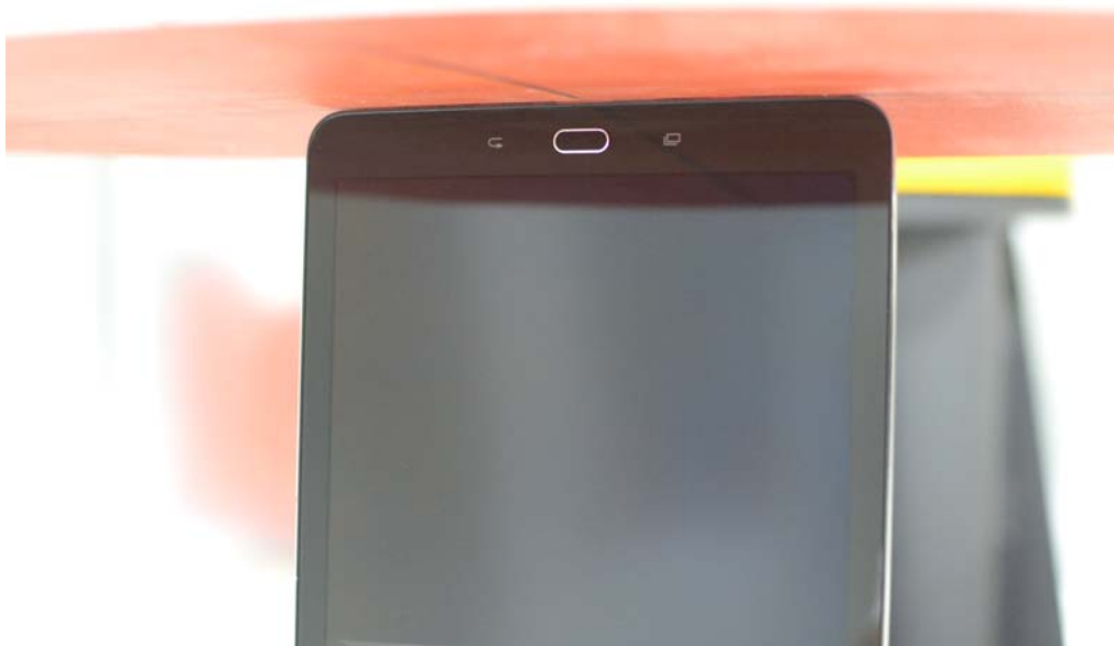
SAR Test Setup Photo 6: Bottom Edge 0.0 cm
