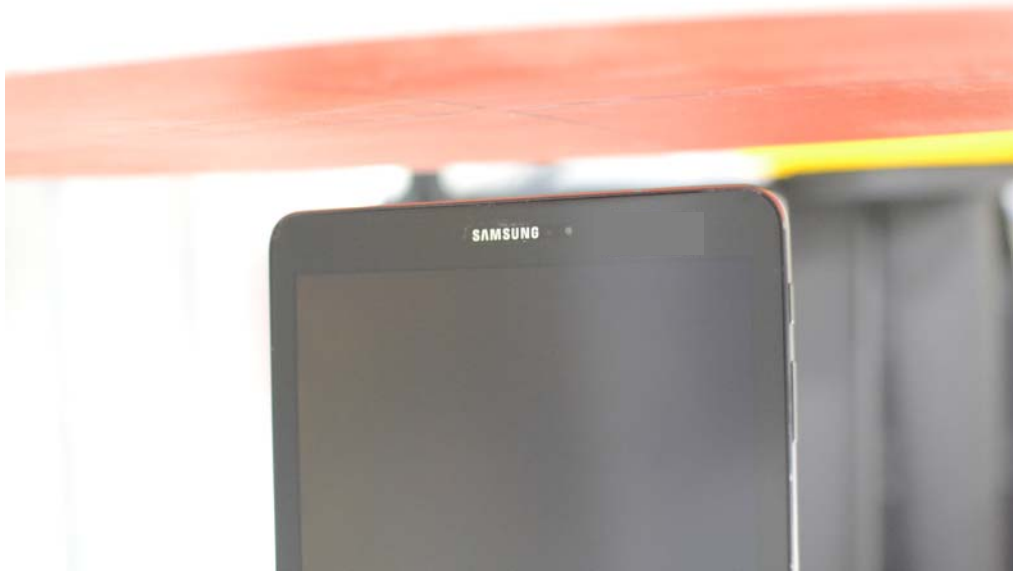
SAR Test Setup Photo 5: Top Edge at 2.4 cm
