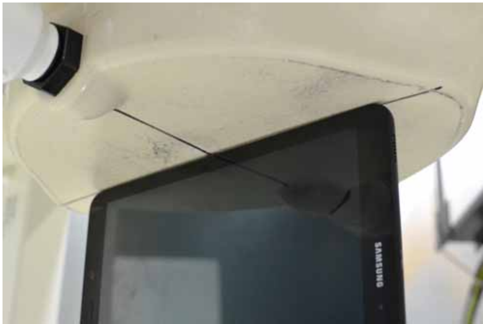
SAR Test Setup Photo 4: Left Edge at 0.0 cm
