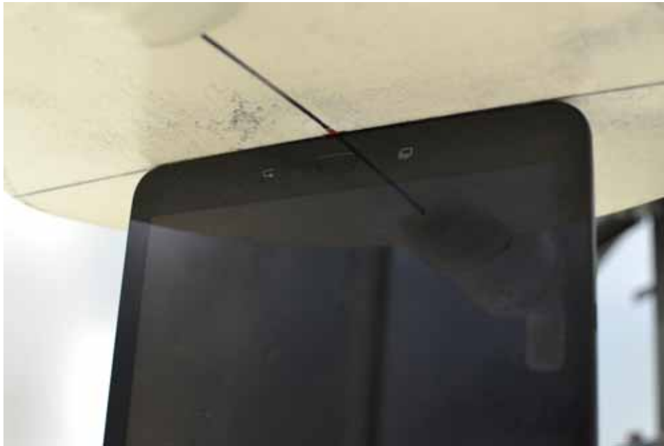
SAR Test Setup Photo 2: Bottom Edge at 0.0 cm
