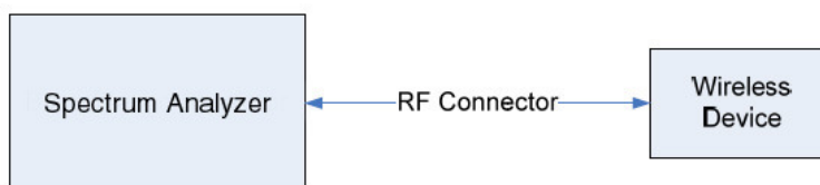
Figure 7-1. Test Instrument & Measurement Setup
