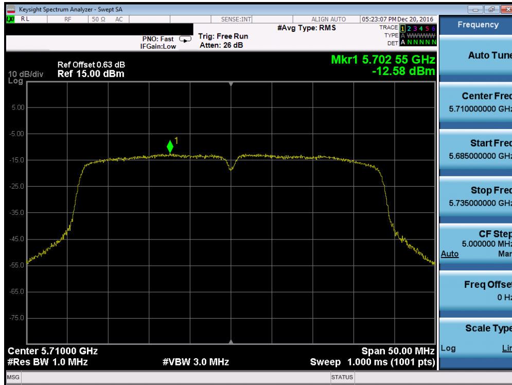
Plot 7-105. Power Spectral Density Plot (40MHz BW 802.11n (UNII Band 2C) – Ch. 142)
